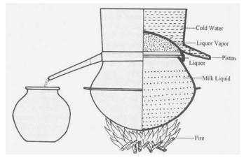
Fig. 3 Reconstruction of the workflow of a bronze still unearthed from Qinglong County (from Luo Xin 2008, 69, fig. 5)
